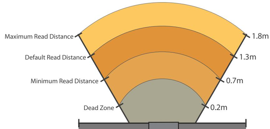
Radar detection range. Spanning from a 60° FOV from the e-loop, these are the range zones. The gray area depicts the dead zone, in which objects cannot be detected. The Minimum read distance is 0.2m. The default read distance is 1.8m, and the Maximum read distance spans up to 2m.
