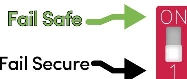
In fail safe mode, if a connection is lost or a low battery is detected the relay will latch on, you can unlatch the relay by pressing the **CODE** button. Low battery is indicated by the continuous flashing of the yellow Menu LED.
