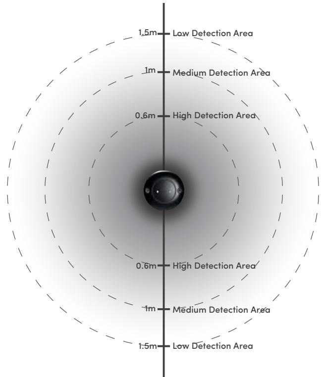
Varying magnetic field detection zones. The grey area depicts a 1m high sensitivity detection area surrounding the e-loop, suitable for the majority of vehicles. The dark colour area depicts a 1.5m medium sensitivity detection area surrounding the e-loop, suitable for most vehicles. The light colour area depicts a 2.5m low sensitivity detection area surrounding the e-loop, which is only suitable for some vehicles.
